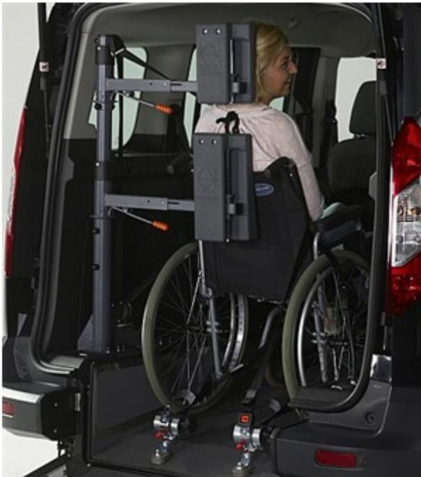
AMF-Bruns' FutureSafe head and backrest, shown here, is designed to help ensure passenger security in a collision.
