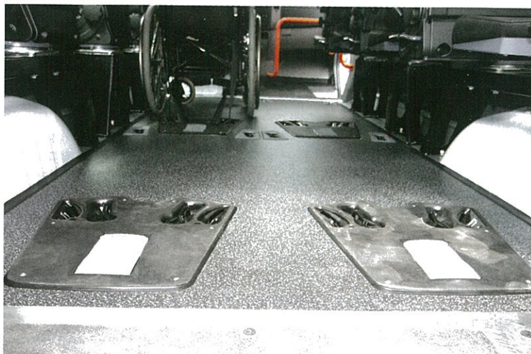
(left) AMF-Brun's PROTEKTOR wheelchair and occupant restraint system provides critical stabilization for passengers in the event of a collision.
