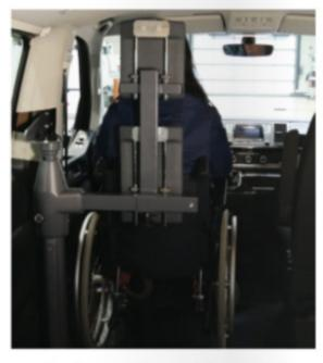
with AMF-Bruns restraint systems, can be turned inward toward the vehicle wall to save space when the vehicle doesn't have a wheelchair passenger, and can be either side or floor mounted. The system is also easy to install, move and clean.
