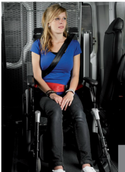
STABLE: Wheelchair restraints, such as these by AMF-Brunns of America, are a must for keeping travelers safe.
